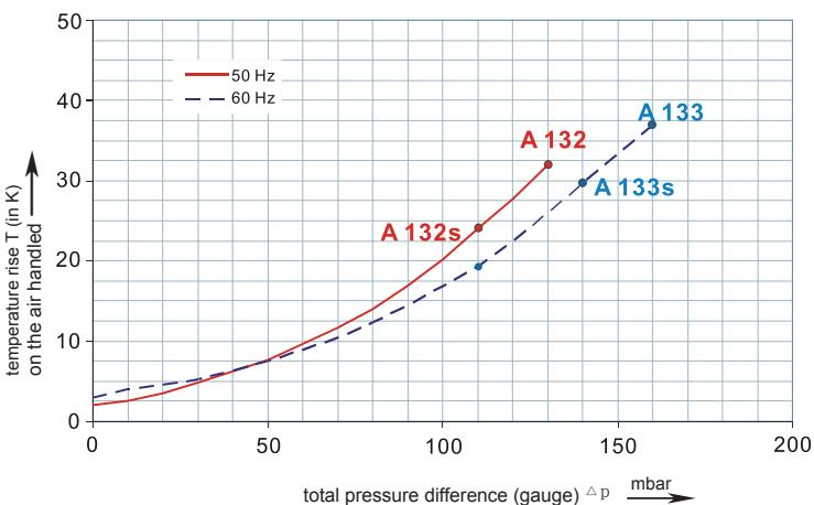
The performance curves are based on air at a temperature of 15 °C and an atmospheric pressure of 1013 mbar with a tolerance of +/- 10 %.
